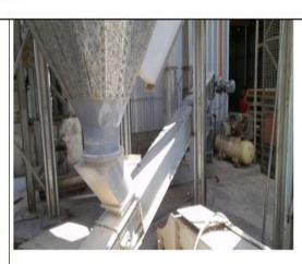
Finish Elevator - The discharged feed from the bottom silo drag is 23 elevates the product and discharges it to the 2way valve.
