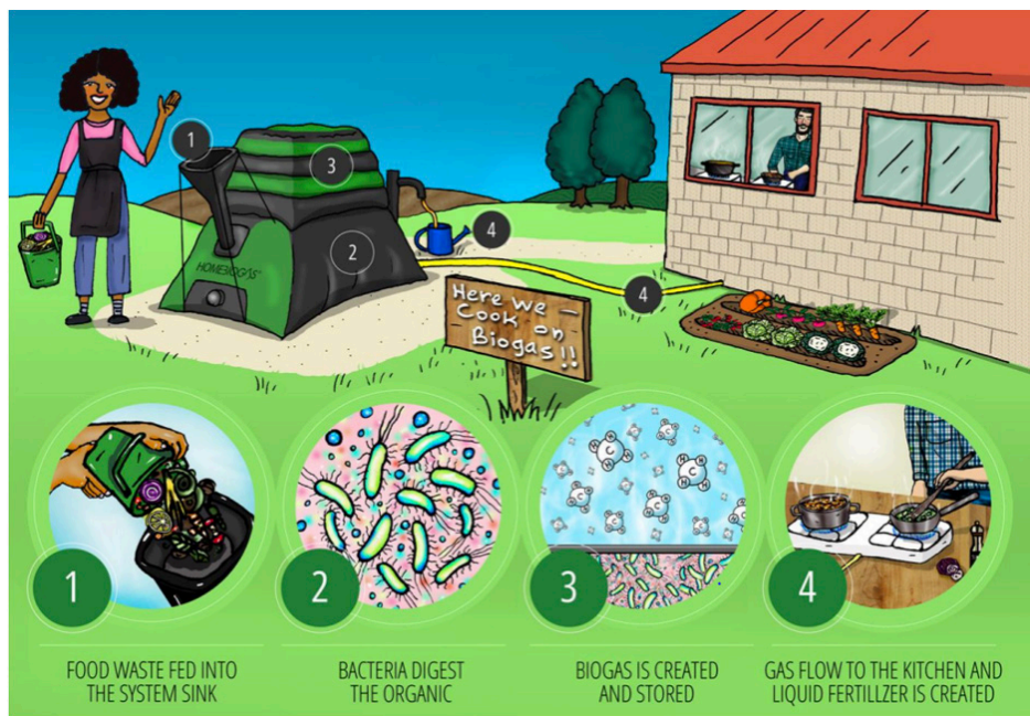
Figure 1: Steps to turn food waste into biogas [2]
